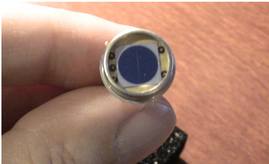
Fig. 1: A 4-Quadrant Photo detector from First Sensor (formerly Pacific Silicon) QP50-6-TO8
