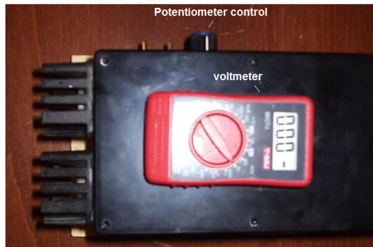
Fig. 8: Picture of the laser potentiometer control and the voltmeter on the enclosure.
